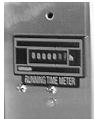
*Running time meter with lamp LED indicator.*
