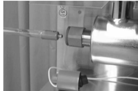
Step 5: Insert lamp into quartz sleeve.
