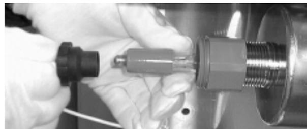
Step 8: Slide boot onto lamp socket assembly.
