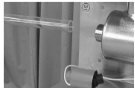
*Insert quartz sleeve into threaded nipple.*
